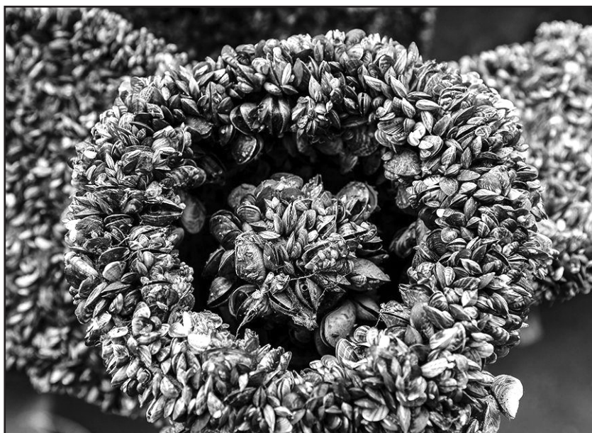
Invasive quagga mussels covering hydroelectric systems on Lake Powell.
