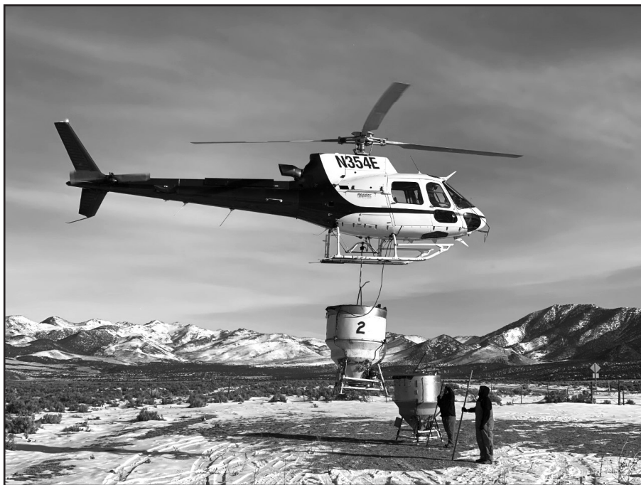
The helicopter lifts off with a broadcast seeder attached. (photo by Kellie Dobrescu)
