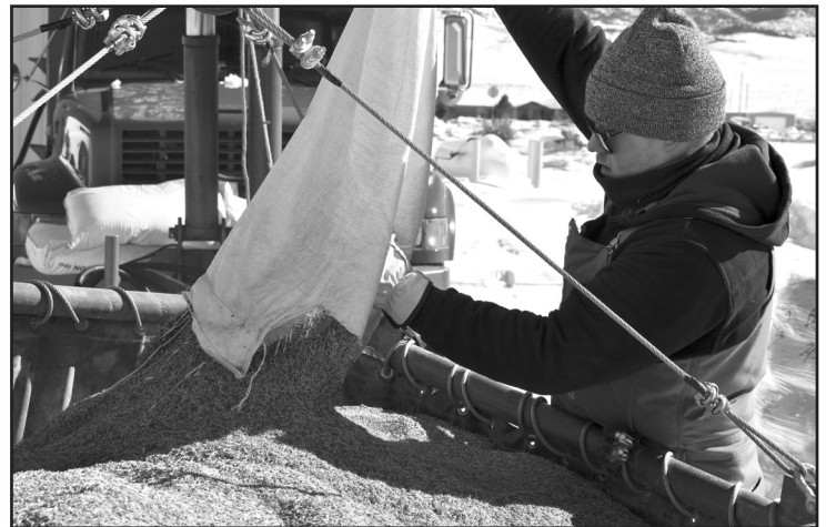
(left) A boom truck operator lowers the filled bag within inches of the hopper of an Air Tractor 802, which can carry up to 800 gallons of seed.
