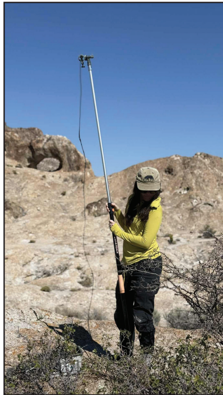
ENLC's Ecologist, Kelsey Danielson, deploying a bat detector in BARNM, with the ultrasonic microphone affixed to a tall painter's pole.
